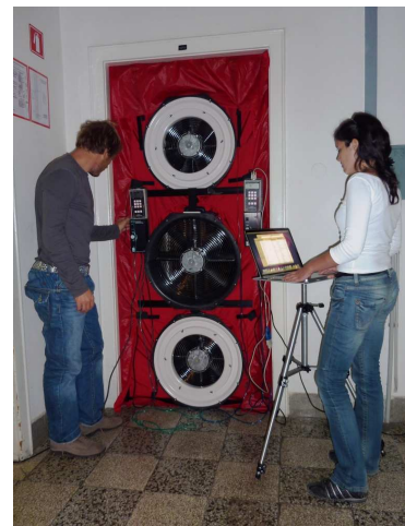
Figure 16: Preparing the blower-door test (BCEI ZRMK)
